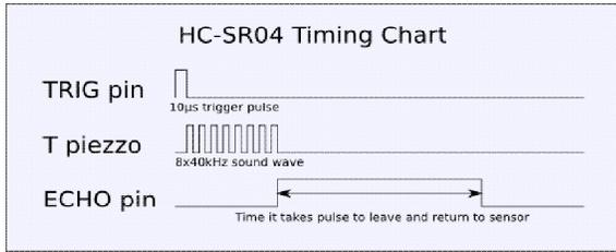
Figure 6 -Ultrasonic sensor timing diagram
