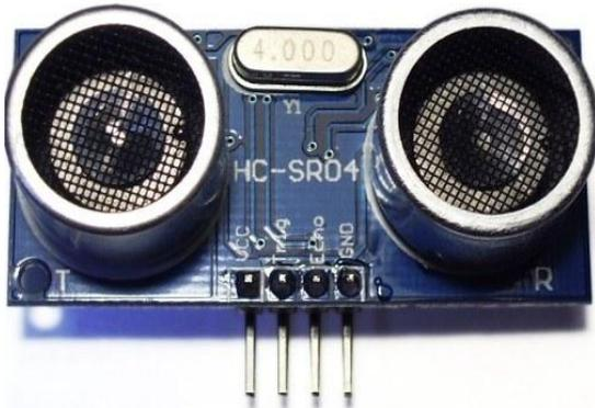
Figure 7- Pin Diagram of Ultrasonic sensor
