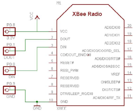
Figure 8-XBee module interfaced with microcontroller
