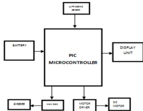
Figure 4- Receiver section
